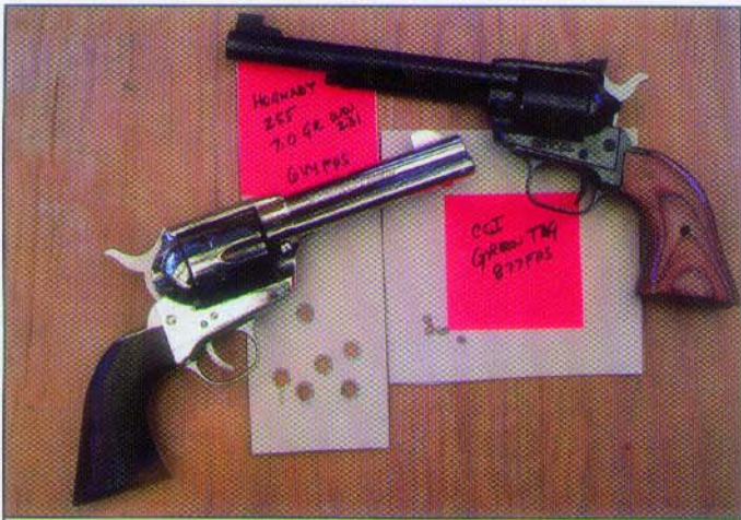
The Heritage Rough Rider .45 Colt is right on for windage and can be brought to point of aim with a little judicious file work on the front sight; the .22 Rough Rider shoots superbly well and can be brought to point of aim using the adjustable rear sight.
